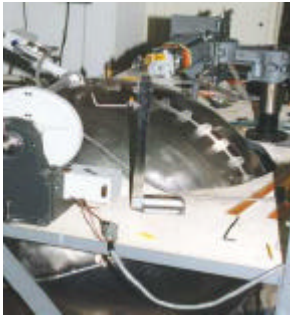
Fig. 2 (on the right)- Prototype of X ray diffractometer realized by Univ of Pisa in collaboration with ISPESL. It's the first mobile diffractometer equipped with height freedom degrees and pointing devices controlled at distance through computer. Within the X-ray adopted optics it gives results equivalent to lab equipments. Tests on different types of materials give good results. Respect the lab diffractometers there is no need to link mechanically the goniometer centre to the specimen holder. The configuration is a virtual centre diffractometer. (Patent just published and at the nationalization stage).
